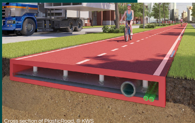
Cross section of PlasticRoad. © KWS
